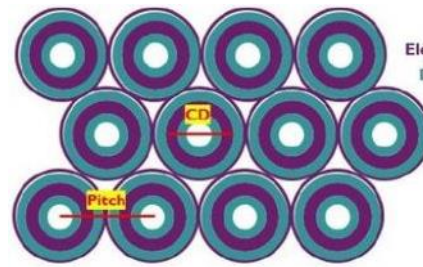
Cup Capacitor Cylindrical (CD: 38 nm~)
